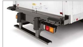
Structural DOT underride & wood filled dock bumper
