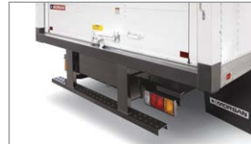
Standard 5" structural DOT underride with poched surface (no dock bumper)
