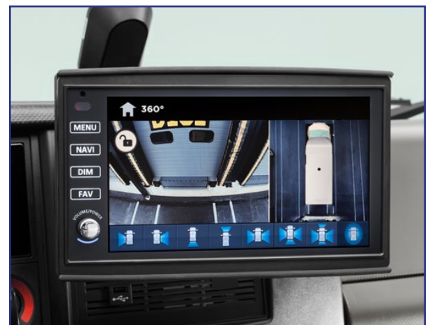
EXTERNAL 360° & INTERNAL CARGO AREA CAMERA
