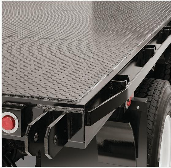
Morgan recognizes the assault heavy-duty haulers may have to endure. That's why they designed in features such as -- structural outside rails for added platform strength, heavy-duty formed steel stake pockets, and steel rub-rails welded over side stake-pockets -- to mitigate downtime, and help ensure that your MHP performs time and again!
