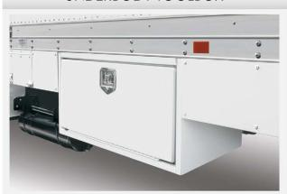
Morgan's optional underbody tool box supports quick and easy access to the equipment you need; and keeps tools out of the cab and cargo areas where they can cause damage.
